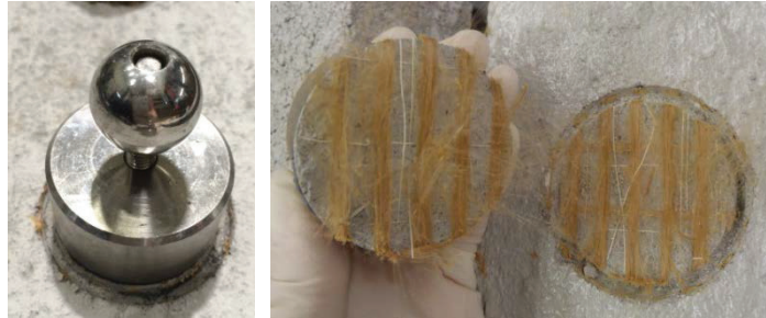
Figure 37 – Bond Strength Typical Failure Mode
