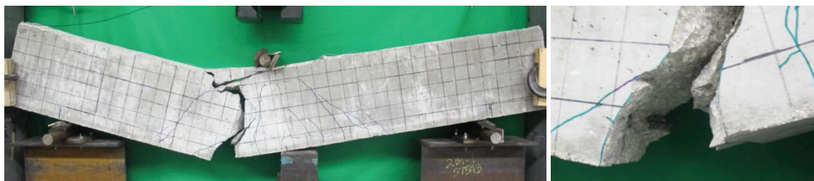
Figure 101 – Typical Fatigue Failure Mode for Unstrengthened RC Beam
