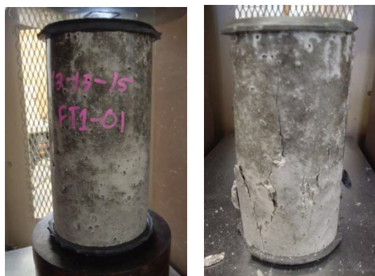
Figure 75 – Concrete Cylinders Before (left) and After (right) Compression Tests
