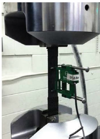
Figure 44 – FRP Tensile Test Setup
