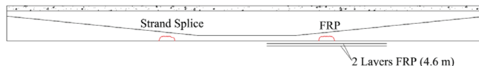
Figure 52 – Girder C FRP Strengthening Configuration
